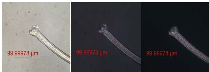
Figure 2: Polyester fibers damaged with a nail gun viewed under plane polarized light (left), 65° crossed polarizers (middle) and 90° crossed polarizers (right). Magnification x400.
