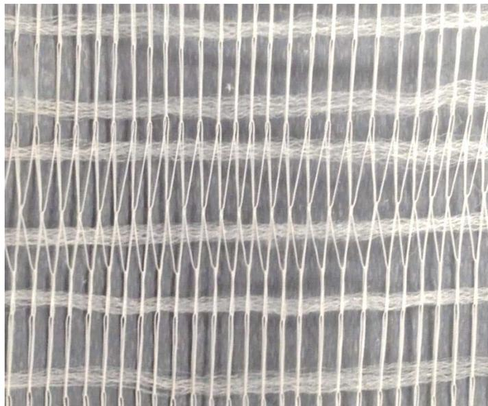
Figure 2: Tricot scrim pattern in IPG duct tape rolls 32, 33, & 38. (machine = 4†, fill = 5↵).
