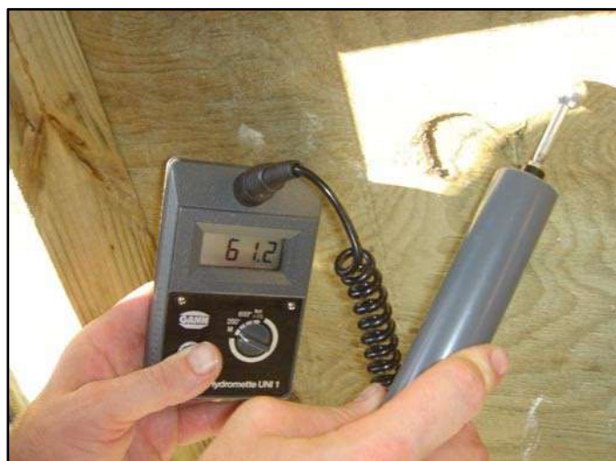
Figure 3b. A non-intrusive/non-penetrating moisture meter-- recommended for initial and interim moisture readings.
