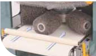
The movements are two by two synchronized to each other. It makes the operation of the machine easy: The operator has only to set the speed of the brushes and the speed of the conveyor.
