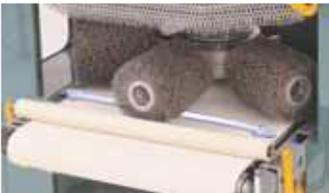
During the process, the entire head and the six spindles rotate and oscillate across the surface of the parts, which means that the processing of the surface is applied from every possible direction, no matter how the part is placed on the conveyor belt.
