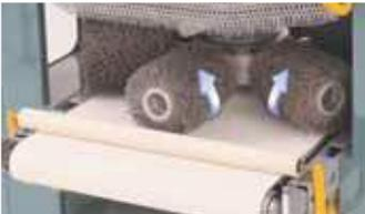
The strong, compact gear head is equipped with a total of six spindles, mounted in pairs, rotating alternately clockwise and counter-clockwise.
