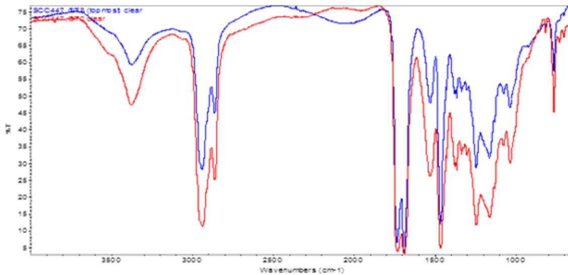
Figure 6: FTIR spectral overlay of two of the four OEM clearcoats (OT2, red; and OT8, the topmost clearcoat, displayed in blue) described in Figure 5. The consistency of the spectra confirm the visual indicators described for Figure 5 that demonstrate no physical or chemical differentiation between the lowermost and topmost clearcoat layers.
