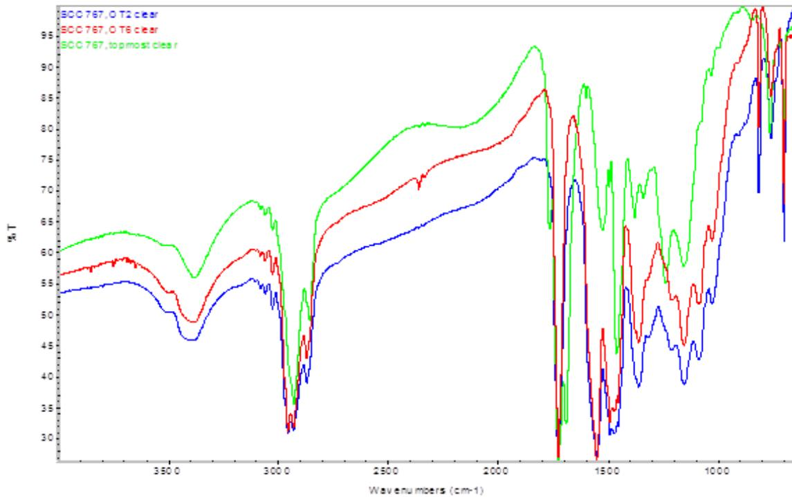
Figure 8: FTIR spectral overlay of the two OEM factory repair clearcoats (OT2, blue and OT6, red, each depicting strong melamine peaks at  $\sim 1550\text{ cm}^{-1}$  and  $\sim 815\text{ cm}^{-1}$ ) for the sample described in Figure 7. The green spectrum indicates that the topmost layer is a polyurethane-based aftermarket refinish (RT1).
