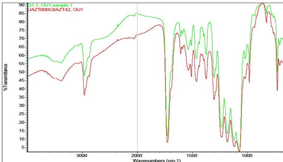
Figure 4. Comparison of the primer surfacer layer from the case sample versus a PDQ sample.
