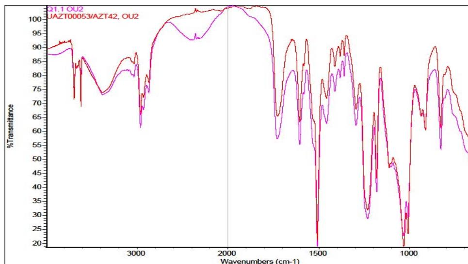
Figure 5. Comparison of the electrocoat layer from the case sample versus a PDQ sample.
