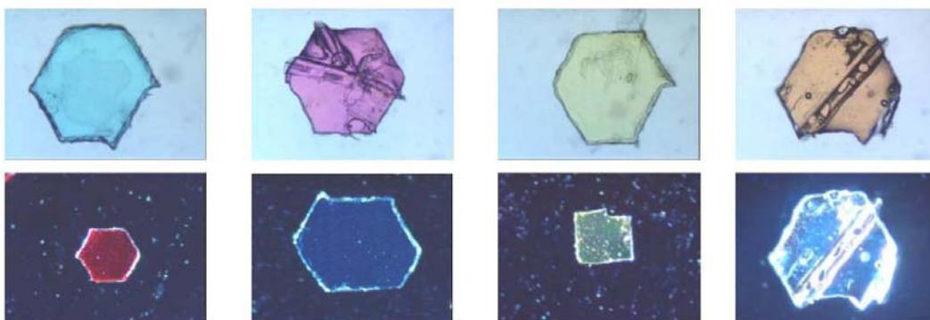
Figure 1: The top row photographed with transmitted light. The second row was photographed with reflected light. It should be noted that the last piece of glitter in the first row is the same piece as the last piece of glitter in the second row—the first under transmitted light and the second under reflected light. All photographs were taken at 100x.
