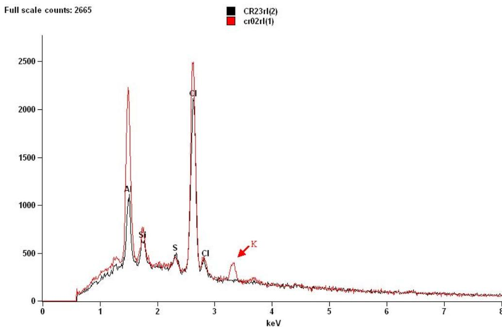
*Figure 6: Spectra from SEM-EDS illustrating the differences in elemental composition from two red pieces of glitter. These pieces of glitter could not be differentiated by physical characteristics (color, shape, size, layer structure) or polymer type (polyester).*
