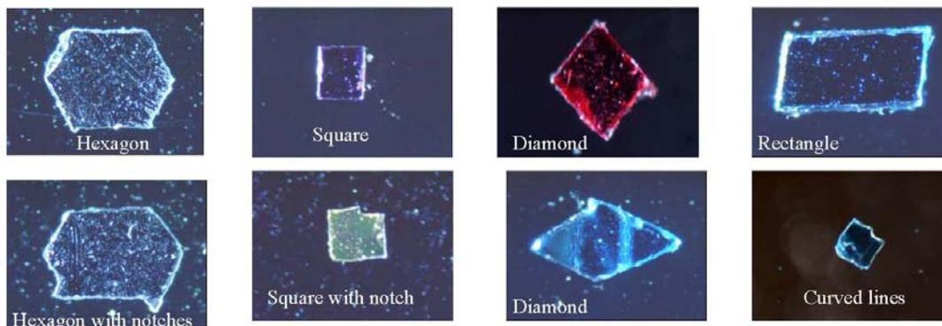
Figure 2: The variety of shapes found in the glitter samples included hexagonal, square, rectangle, and diamond/rhombus. Some samples included notches or curved lines. Photographs were taken at 100x with reflected light.
