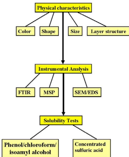
Figure 10: Analysis scheme for the examination of glitter. Since the solubility tests are destructive, they are left for the last step of the analysis scheme.
