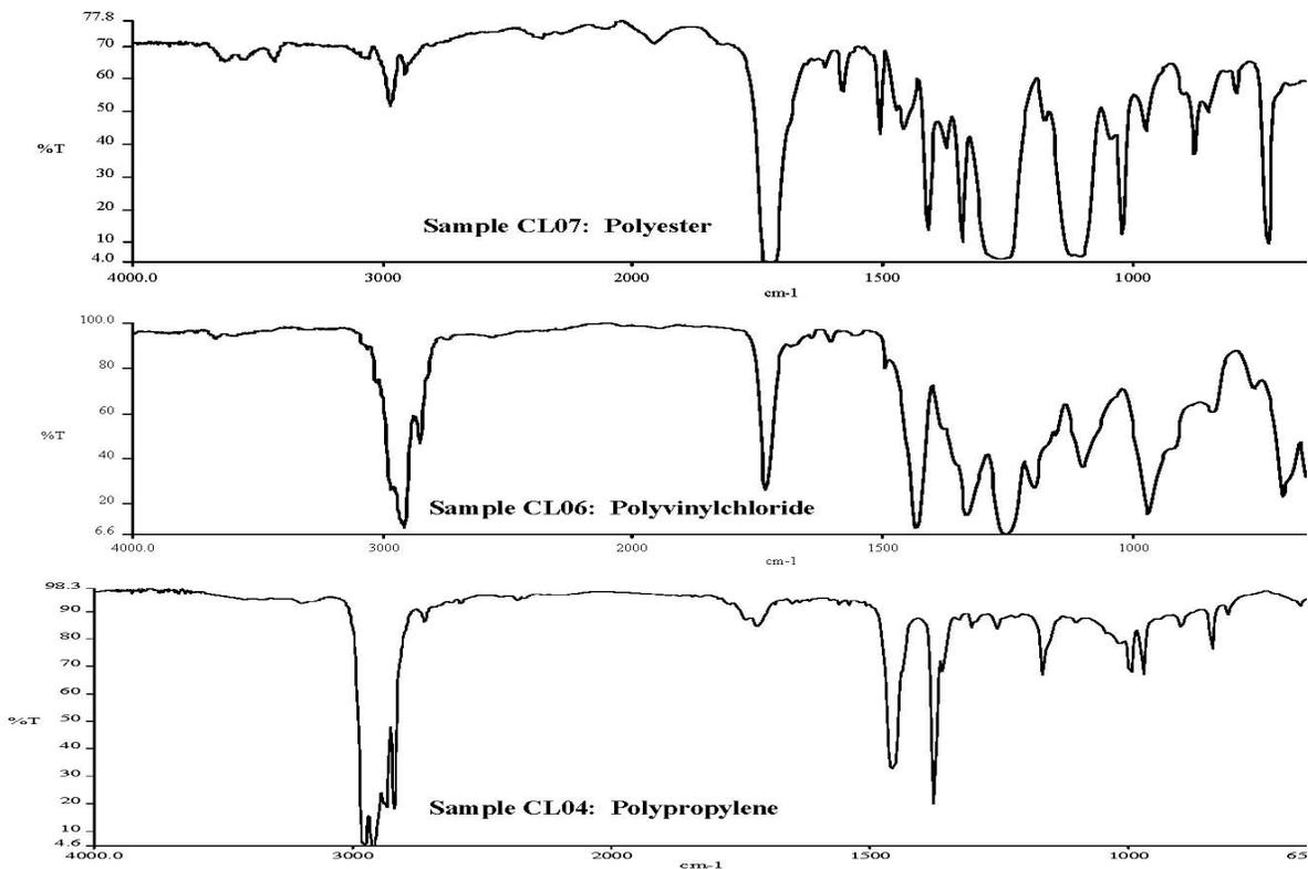
Figure 5: Three different polymer types as determined by FTIR.
