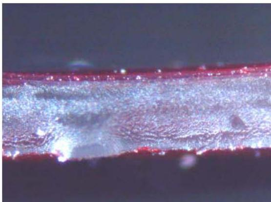
Figure 8: Cross-section of a piece of red glitter illustrating the 3 layer structure (red, clear, red) under a PLM with reflected light.
