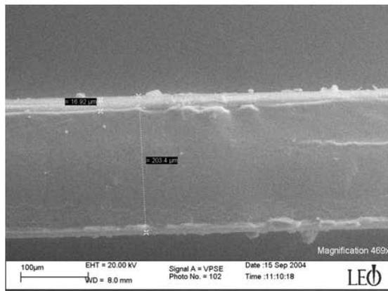
Figure 9: Cross-section of a piece of red glitter illustrating the 3 layer structure (red, clear, red) under the SEM.
