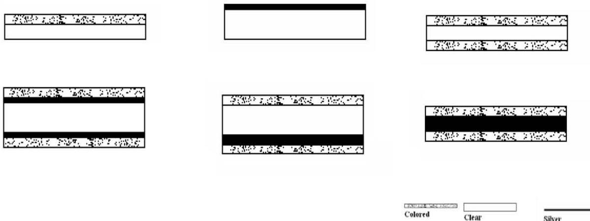
**Figure 3:** Some of the different layer structures that were found among the glitter samples. The structure varied from one to five layers.
